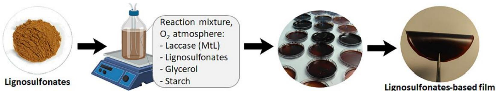
**Scheme 1.** Summary of the process steps for synthesizing lignosulfonates-starch films by laccase polymerization.
