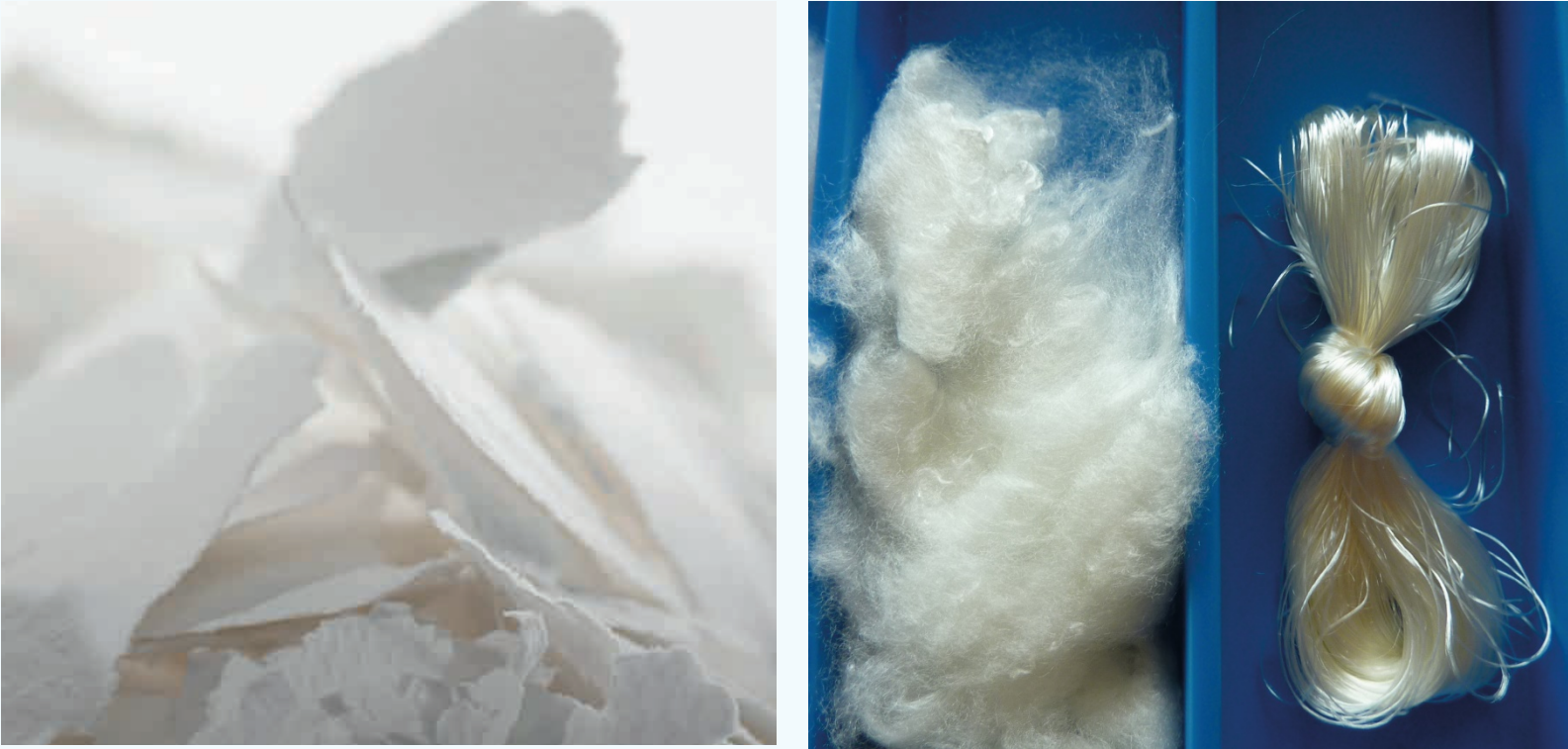
Left: pulp cellulose (photo: Lenzing)/ right photo: spun fiber (left) filament yarn (right)
